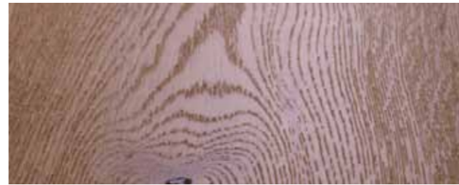
Lacquer sits on the surface of the timber after the soft grain has been brushed out of the board
